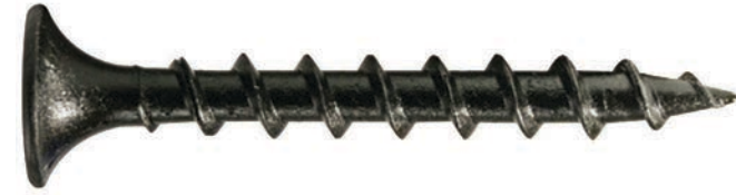
BUGLE HEAD PHILLIPS COARSE THREAD DRYWALL/WOOD SCREW, BLACK PHOSPHATE
